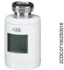
The Valve Drive EnOcean is used for efficient control of room temperature in private and commercial facilities. It communicates wirelessly via a bidirectional EnOcean standard radio protocol, and it features a large display and a rotary knob for manual operation. It is powered by two 1.5 V AA lithium batteries. The Valve Drive EnOcean is suitable for use with the ABB i-bus KNX KNX/EnOcean Gateway EG/A 32.2.1).
